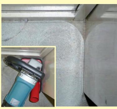
The Corner Shroud design allows grinding and polishing into a corner with no dust problem as easily and tightly as if there was no shroud at all.
