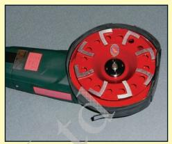
3. Use the nut provided with your grinder to secure the disc in place. Adjust the seal with a slight gap between the seal and the floor. On rougher surfaces the seal can be fitted closer to the floor for a better dust seal or when using high powered vacuums it can be lifted to allow a larger gap to prevent suck-down.
