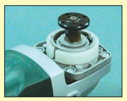
1. Fit the appropriate insert over the grinder mounting boss with the gap facing the body of the grinder. Place the shroud over the insert and lightly tighten the three screws to position the shroud. When you are sure the shroud is on straight and the disc fits correctly then tighten the screws hard so they thread into the plastic insert.
