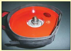
2. Place 3 to 6 spacer washers directly onto the grinder shaft so that the disc when fitted will not make contact with the shroud edging plate or the shroud body. Ideal clearance is 2mm to 5mm between the disc and the edging plate. If this is difficult to achieve further adjustment can be made by moving the shroud up or down on the mounting boss of the grinder before fully tightening the three screws.
